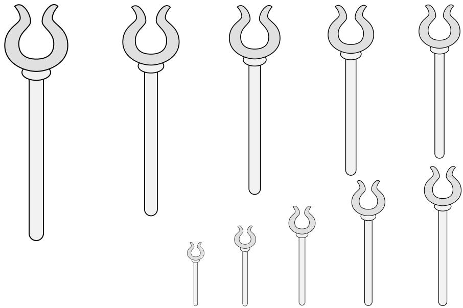
A pivoting pin with a forked head used to secure oars to the side of a boat.
