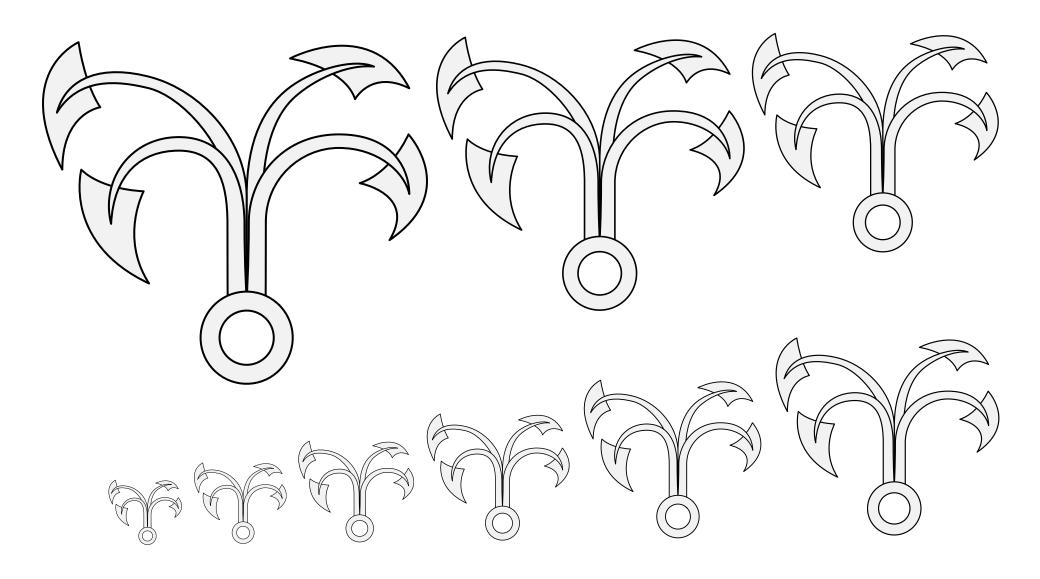
A device similar to an anchor, but with additional hooks, used with a rope to drag or catch something.
