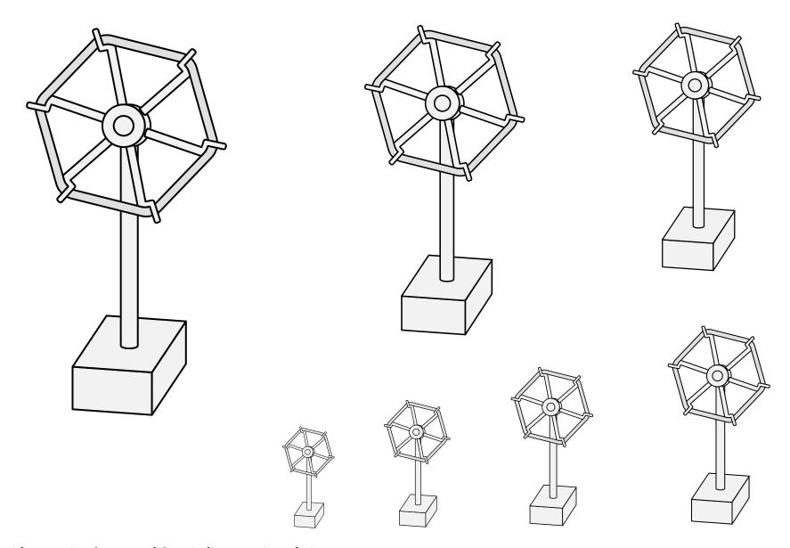
A stand with a rotating frame used for winding yarn into skeins.
